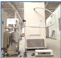
LN 2 /CO 2 backup system
